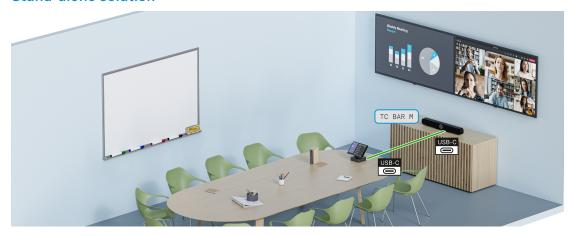
The TC Bar is connected via USB-C® directly to a notebook or or via other UVC- and UAC-capable USB host devices. There is no need for a network connection. In this mode, only restricted functions are available.
