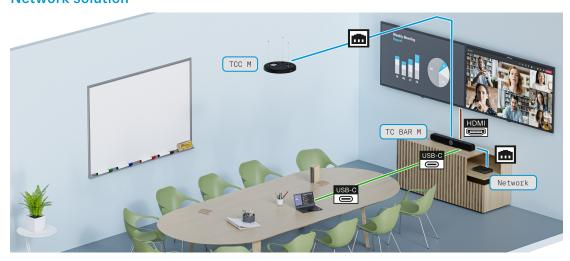
The TC Bar can be connected to an existing network infrastructure and controlled remotely by the Sennheiser or 3rd party control software.
